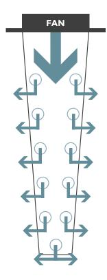
When a fan runs, the air it moves will travel in a straight line unless it is prevented from doing so. In a plenum fitted with a vertical fan, this means air flow is biased to floor level. A 'sock' fitted to the fan (above) reduces velocity pressure generated by output from the fan and, instead, builds static pressure within the sock. With the help of correctly sized and spaced outlets and a tapered shape, any vertical airflow gradient can be reduced.
